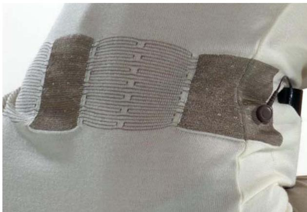
The Mini-Power-Controller and the heating zones are forming an electric circuit around the waist. The conductive fabric is made exclusively from silver plated polyamide so that the resistance is very
